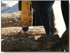
Drilling logs with ordinary drill, note stop collar.
